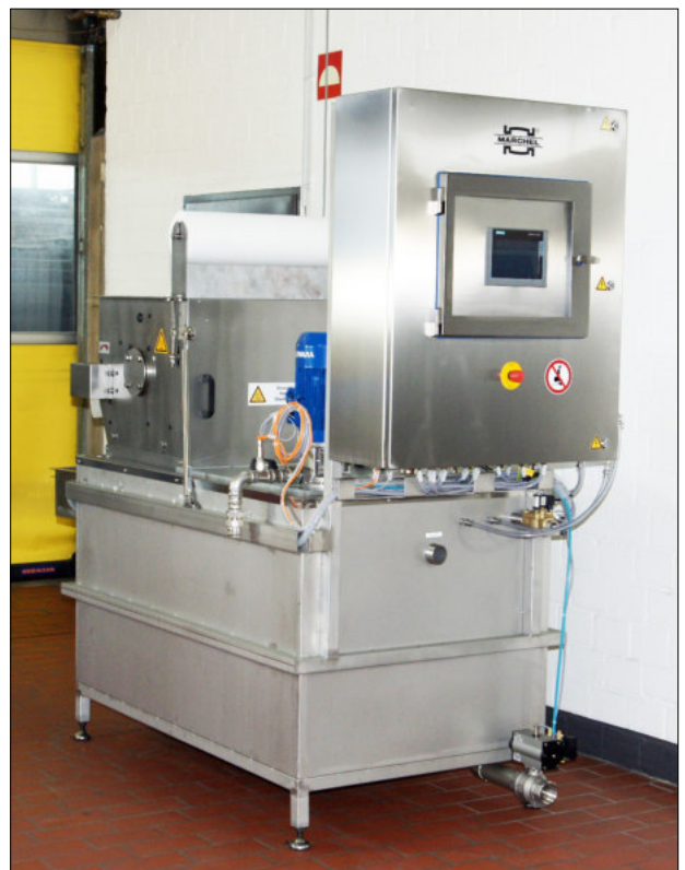
Filtering and control unit with capacity of 550 liters
